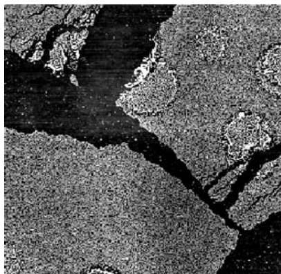
FIGURE 1 (see COLOR PLATE VI) AFM image of a single monolayer of PA4 as deposited at high surface pressure, \Phi = 15 mN/m. Lateral size is 10\text{ }\mu\text{m} , vertical contrast corresponds to 5\text{ nm} .
